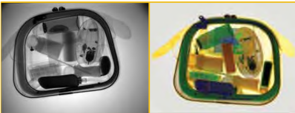
Dual energy option: suspicious articles (in red)
