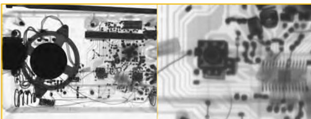
Geometric magnification with microfocus generator
